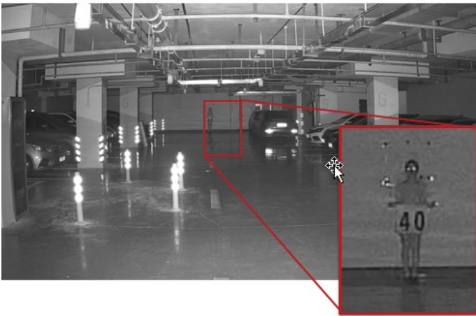
DS-2CD2043G2-I (6mm) Max IR distance: 132 ft. (40mm)
